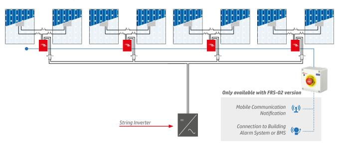
**NOTE:** If two panel installation is used in accordance with NEC 2017, each panel must be <40V. For strings with an odd number of PV panels, single panels can also be connected to IMO FRS-01/02 units.
